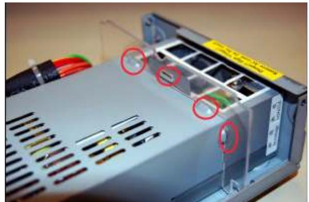
When reinstalling the power supply please make sure none of the cable interferes with the fan or are pinched anywhere else.
