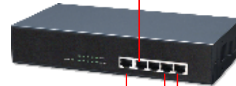
Ethernet Switch (may use integral switch in Router)
